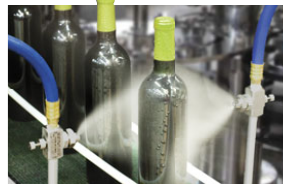
(2) Model EB1030SS atomizing nozzles are used to give a final sanitizing rinse prior to labeling wine bottles.
